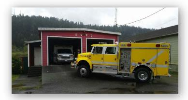
The Department's new Measure Z funded 4-wheel drive fire engine will allow us to access all roads in our district as well as outlying areas. This engine also has a larger pump, which will improve our structure fire suppression capabilities.
